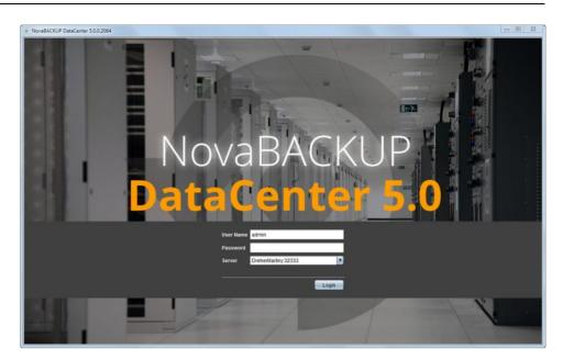
The default setting for the initial login is *User Name admin* and the field for the password is left blank. After you have logged in, you can define the password in User management.
