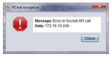
The error message *Error in Socket API call* means that this ID address could not be connected with the TCP connection (stream socket).
